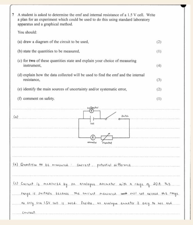
Potential difference across the cell is measured by a voltmeter with a range of 5V. This range is snitable because the ent of the cell is 1.5V so the maximum value of p.d. measured is only 5V.
